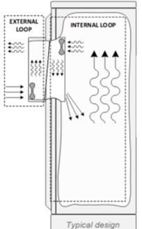
Cooling system does not allow exchange of air between ambient and cabinet interior
